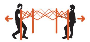
Grab the bottom of the central truss bar (as shown on the picture).
